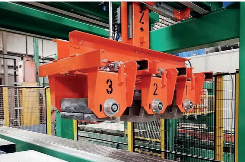
"Cerberus" the programming gripper with three independent heads.
