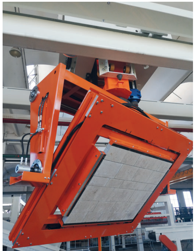
Four axes gripping head with mechanical jaws
