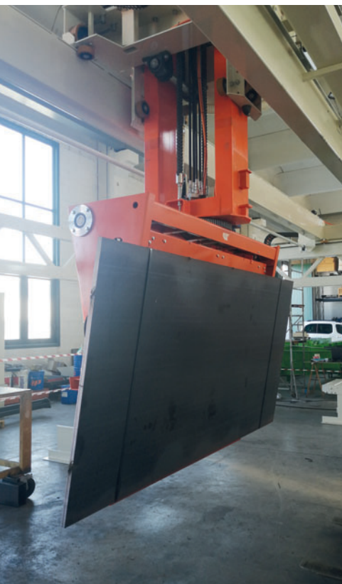
Vacuum gripping head (for tiles)
