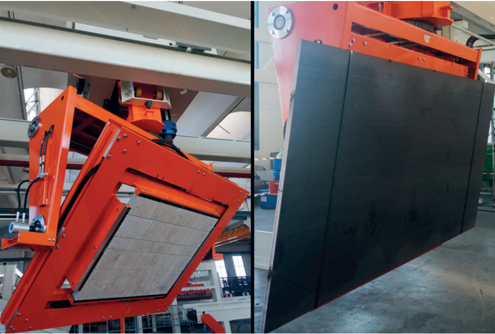
Mechanical and vacuum heads gripping different products
