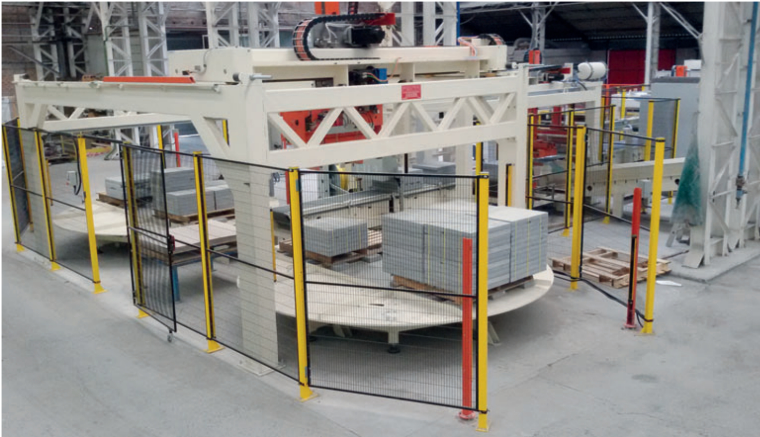
Fig. 6: Stacking gripper with 5 axis and 2 rotating platforms
