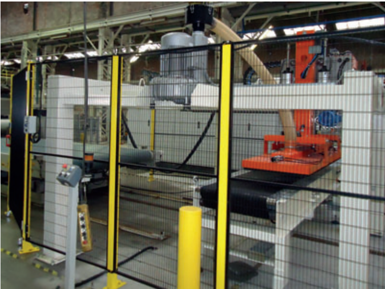
Fig. 2: Gripper with vacuum plate
