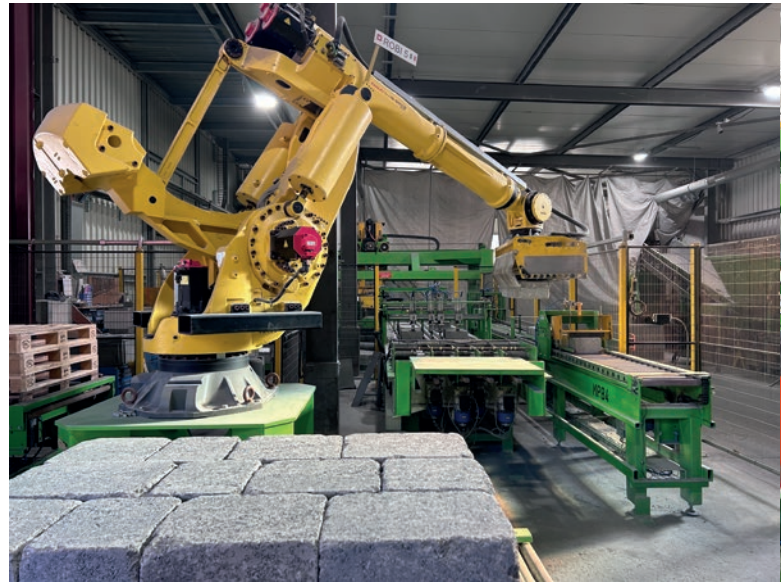
From the programming tracks, the sorted rows of bricks are fed to a FANUC packaging robot. A specially developed gripper picks up the rows and places them on Euro pallets.
