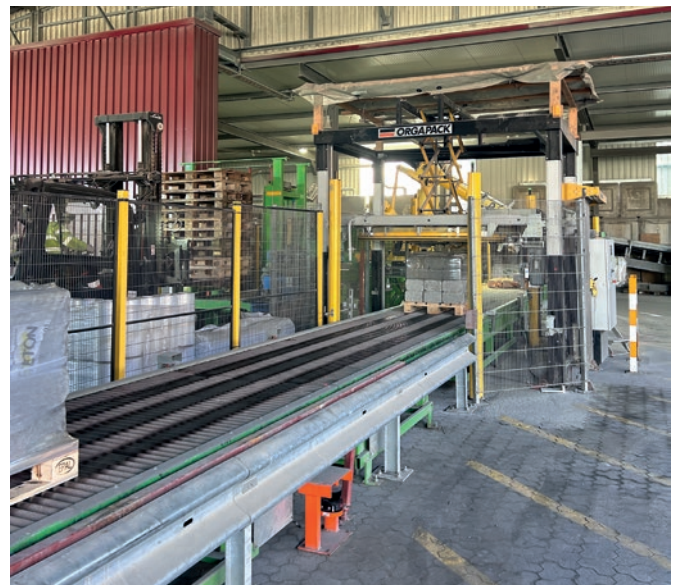
The finished parcels are transported via roller conveyors to the Octopus stretch wrapping machine and then picked up by a forklift at the transfer point.
