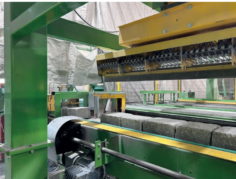
The bricks are fed into the sorting system in strands and transferred by gripper robots.
