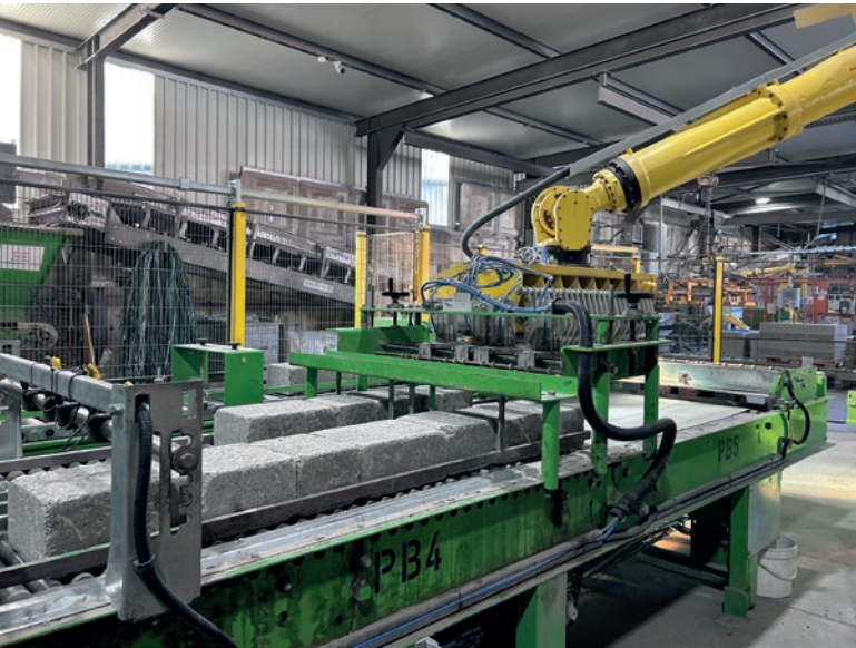
From the programming tracks, the sorted rows of bricks are fed to a FANUC packaging robot. A specially developed gripper picks up the rows and places them on Euro pallets.
