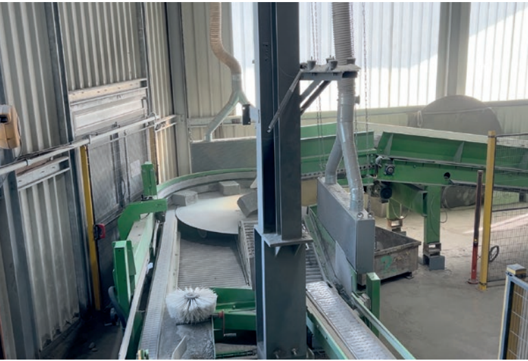
The reinforced turntable directs the products centrifugally to the outer wall, where they are then transferred to the sorter via a conveyor belt.
