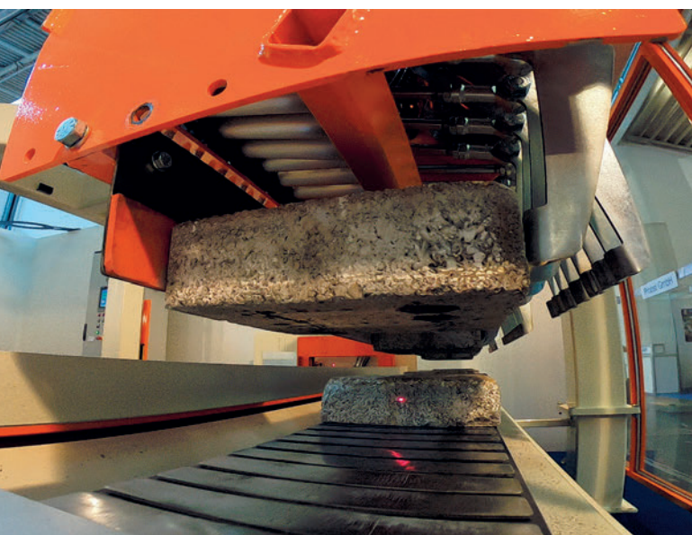
3. Sorting gripper deposits the products
