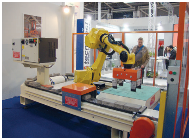
bauma 2013 - Robot scanning system to build preset pattern
