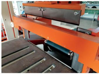
The concrete waste created by the pitching process is automatically ejected and collected on the waste belt placed under the blades position.
